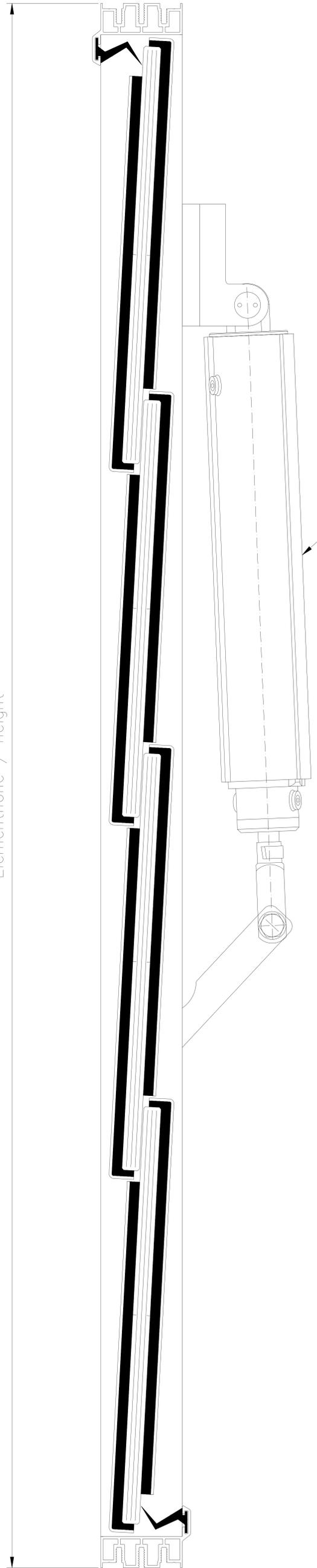
Pneumatikzylinder / pneumatic cylinder
