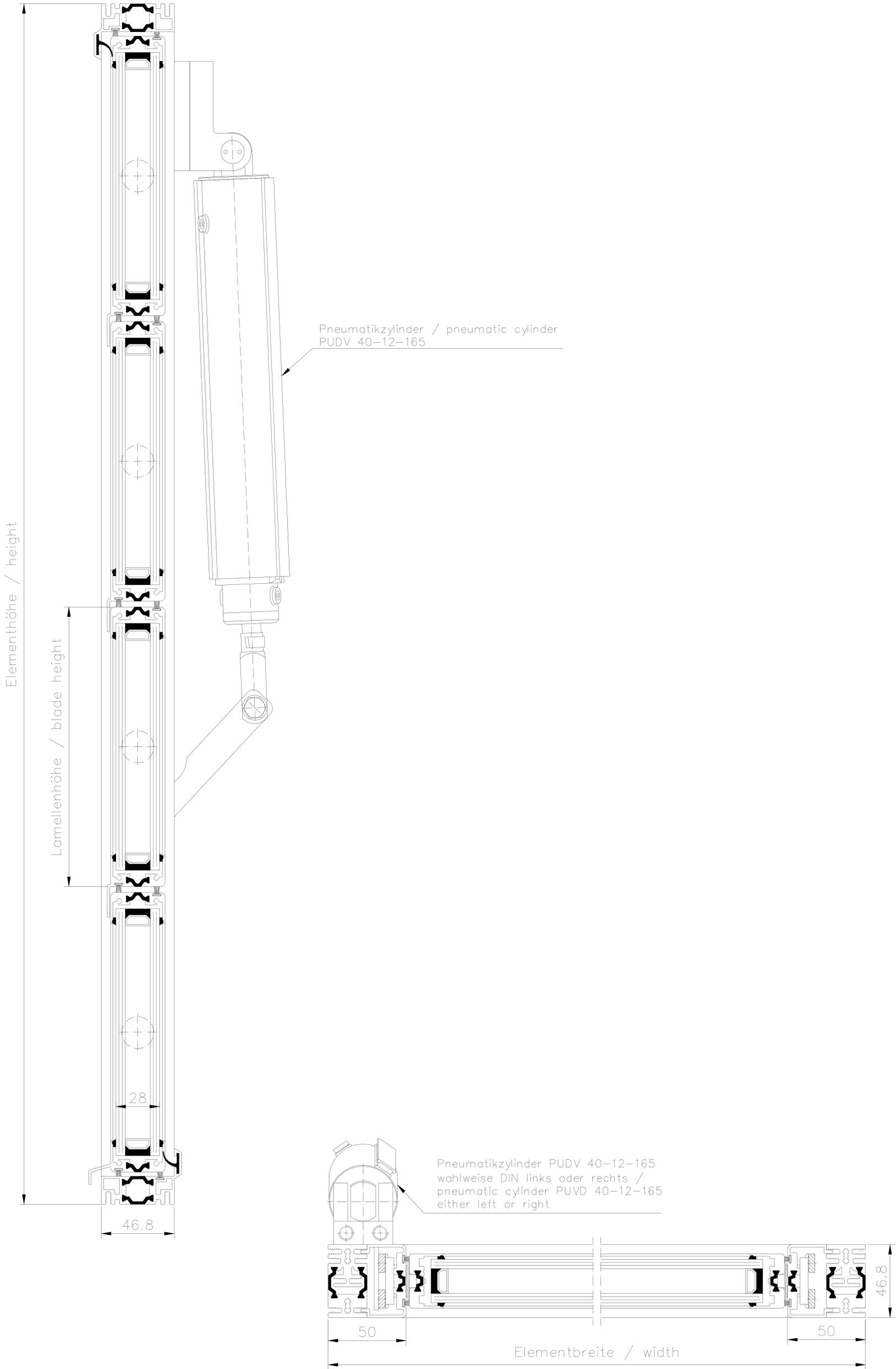
Pneumatikzylinder / pneumatic cylinder
