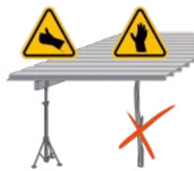
9 ■ Use a suitable prop equipment
