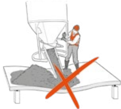
19 ■ Avoid any concrete accumulation while concreting
