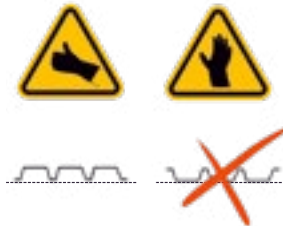
12 ■ Comply with correct orientation of the profile sheet
