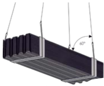
2 ■ Use adequate slings and lifting tools to unload bundles
