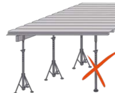
17 ■ In case of propping, use a classical formwork beams instead of single props
