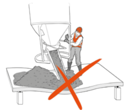
19 ■ Avoid any concrete accumulation while concreting
