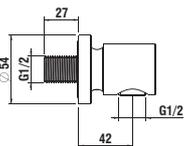
Technical drawing showing dimensions: 27,  $\varnothing 54$ , G1/2, 42.
