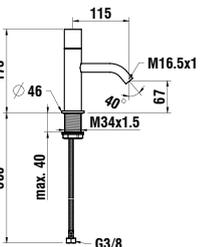
Technical drawing showing dimensions: 173, 115,  $\varnothing 46$ , max. 40, 380, G3/8, M16.5x1, M34x1.5.
