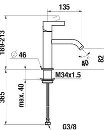
Technical drawing showing dimensions: 189-213, 135, 40,  $\varnothing 46$ , max. 40, 365, G3/8, M16.5x1, M34x1.5.
