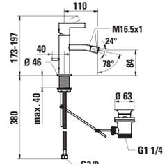
Technical drawing showing dimensions: 173-197, 110, 40,  $\varnothing 46$ , max. 40, 380, G3/8, M16.5x1, M34x1.5, G1 1/4, 24°, 78°, 84.
