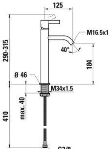
Technical drawing showing dimensions: 290-315, 125, 40,  $\varnothing 46$ , max. 40, 410, G3/8, M16.5x1, M34x1.5, 184.
