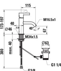
Technical drawing showing dimensions: 173-197, 115, 40,  $\varnothing 46$ , max. 40, 380, G3/8, M16.5x1, M34x1.5, G1 1/4.
